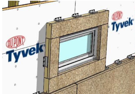
Figure 16. Install window head
