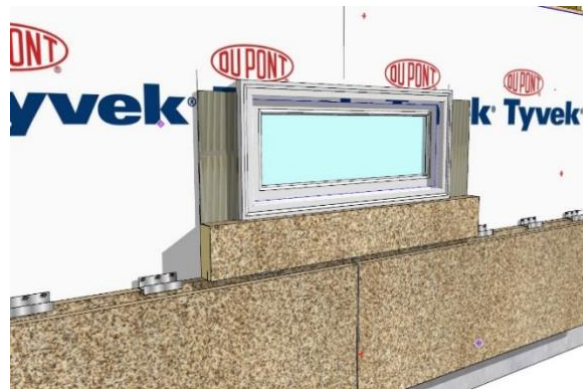
Figure 14. Apply Adhesive for Window Jambs
