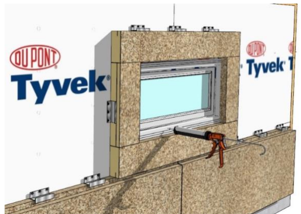
Figure 17. Seal window closures
