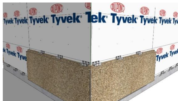
Figure 21. Start from the corner of the wall toward the middle.
